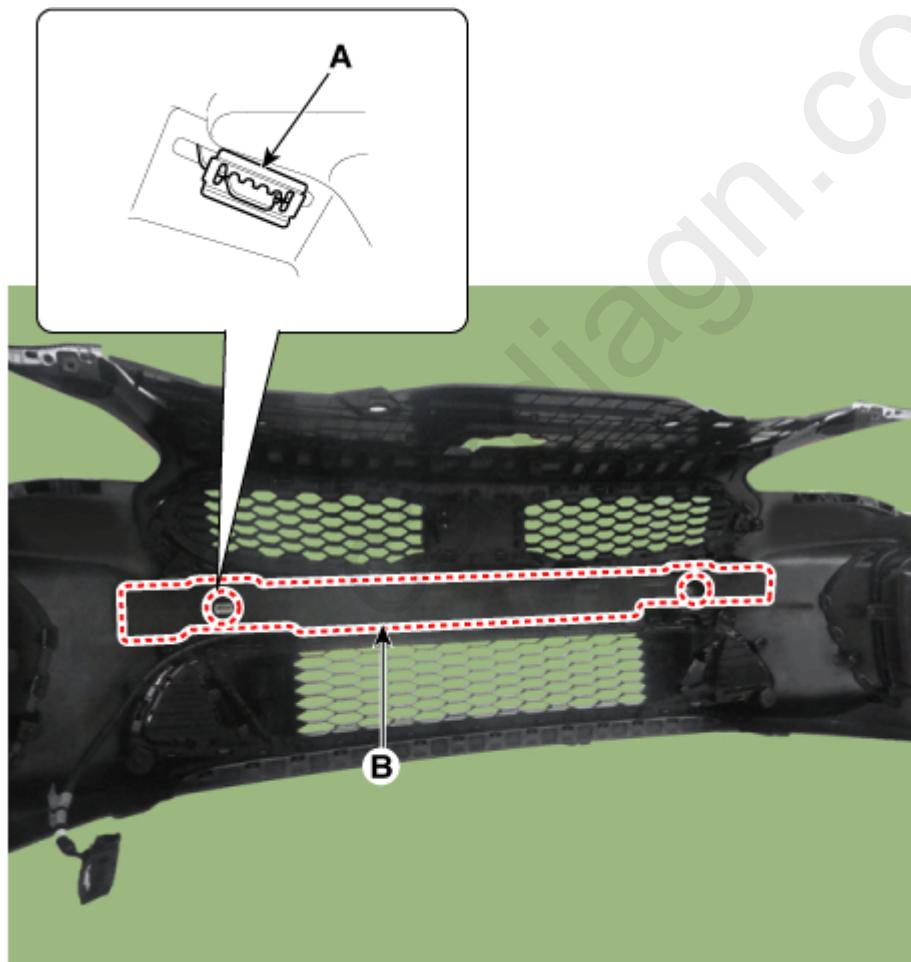
3. Remove the front bumper wiring (A).
