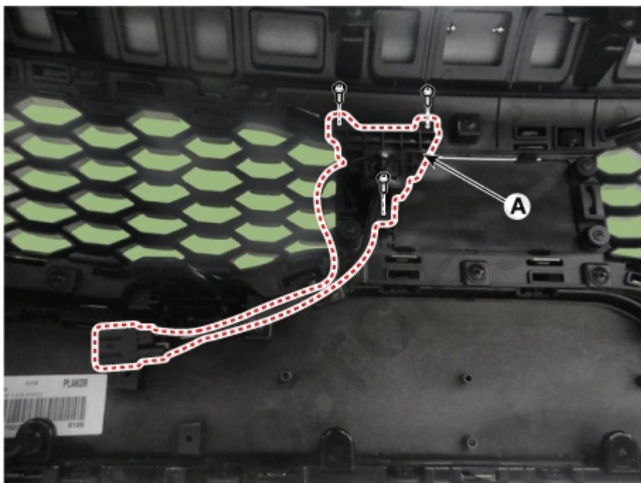
5. Remove the radiator upper cover (A) after loosening the screws.
