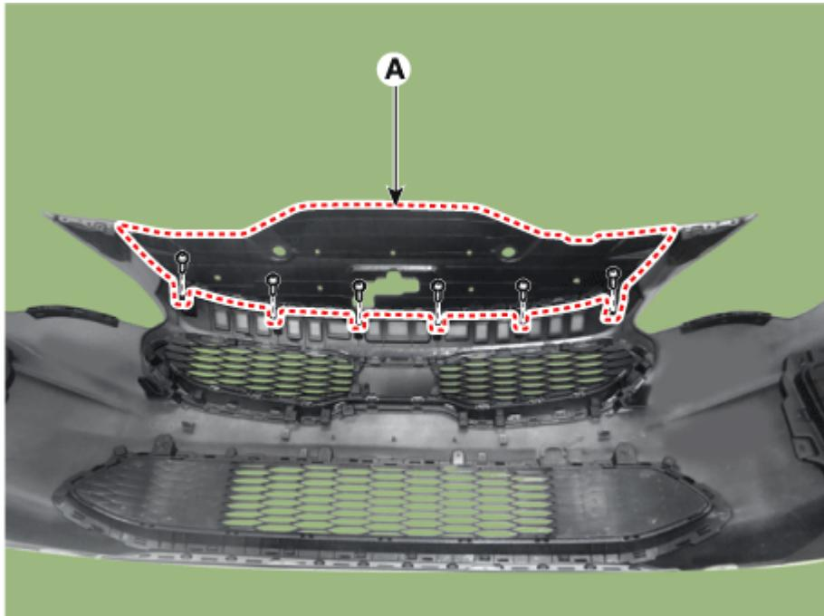
6. Remove the radiator grille (A) after loosening the screws.
